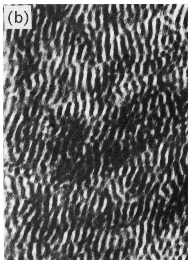
Figure 6. Transmission electron micrographs of annealed specimens (annealed at 160 °C for 12 h) of the cross-linked TR2400 prepared with the concentration of peroxide at 0.5 wt % for (a) through and (b) edge views.
